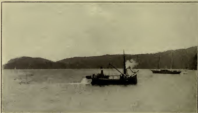
The salvage steamer Bremer equipped with suction dredge, removing a sandbank from the supposed location of the Florencia galleon in 1909.
